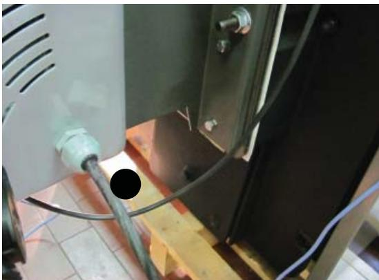
Fig. 37 Connection to the mains
