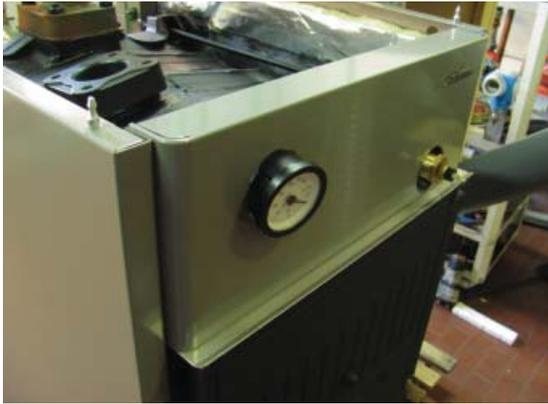
Fig. 29 Remove the thermometer
