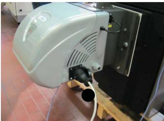
Fig. 33 Screw feeder motor cable
