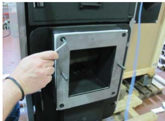
Fig. 23 Plate fixed to the combustion chamber door
